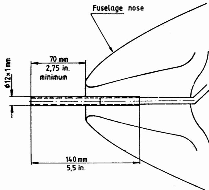
Brass tube 5,5 in = 140 mm in length (12  $\phi$  x 1).
