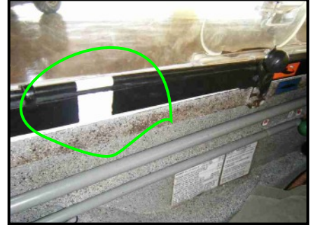
Owl: Front seat canopy latch closed and locked. White over White, You're All Right.
