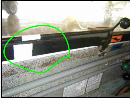
Owl: Front seat canopy latch in motion but not yet closed. This a dangerous condition!
